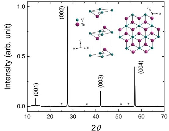
FIG. 1. (color online) X-ray diffraction patterns of  $1T$ - $VTe_2$  single crystals. Asterisks mark peaks that do not belong to the trigonal phase. Inset: Schematic atomic structure of  $1T$ - $VTe_2$ . Olive and purple circles represent V and Te atoms, respectively.
