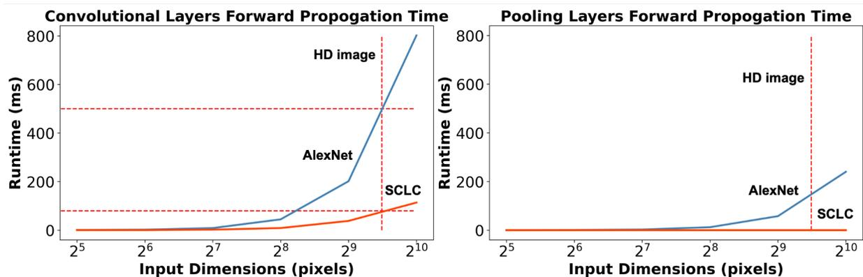
**FIGURE 3.** Comparison of forward propagation time between AlexNet (blue line) and its SCLC (red line). Left: Propagation time through a single convolutional layer for variable image dimensions; Right: Propagation time through a single pooling layer for variable image dimensions. The dashed lines mark the resolution of an HD image and its corresponding runtime in AlexNet and SCLC.
