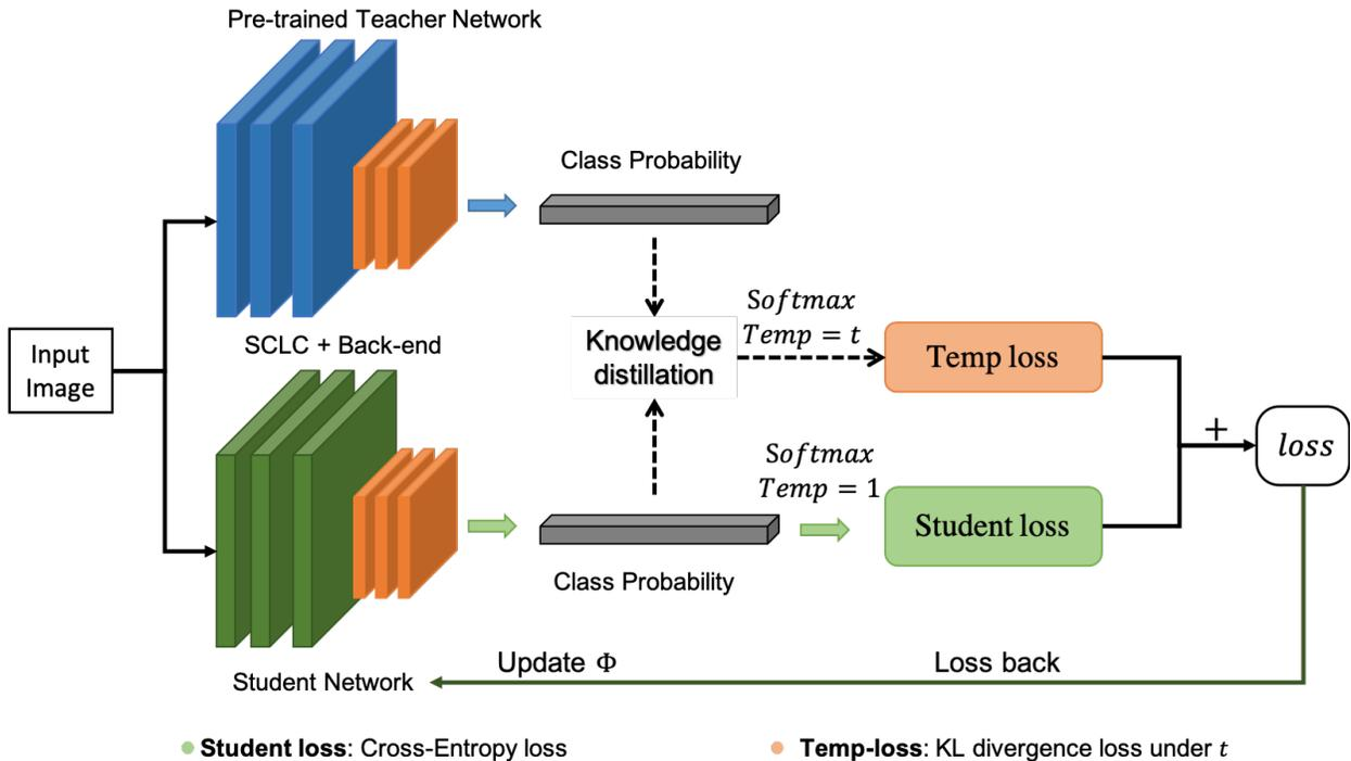
**FIGURE 1.** Illustration of KD training. Student network (green-bottom) parameters  $\Phi$  are updated according to an interpolation of two losses: the Student loss (Crossentropy loss between data and the student model output) and Temp loss (Cross-entropy loss or KL divergence) between the teacher network (blue-top) and student class distribution with a temperature parameter  $T$ .
