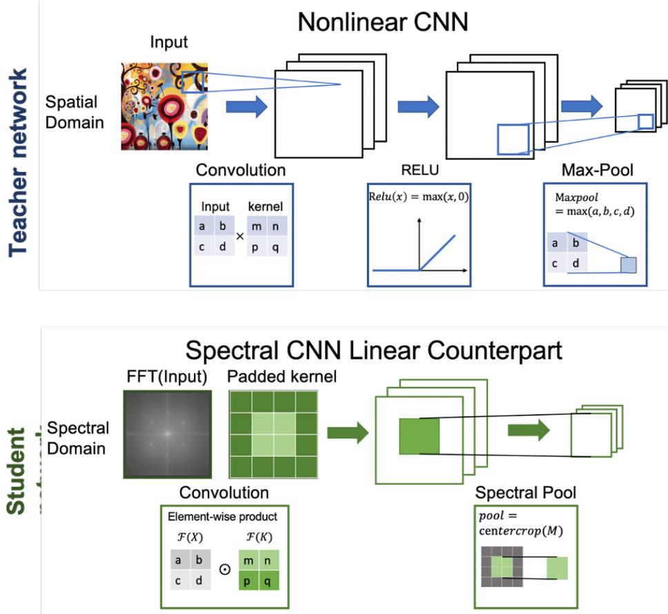
**FIGURE 2.** Nonlinear CNN (top) and the proposed substitute, Spectral CNN Linear Counterpart (SCLC) (bottom). Top: An exemplar nonlinear CNN with layers that include operations of Convolution, Nonlinear RELU activation, and Max-Pool. Bottom: SCLC of the CNN shown in top row. The Convolution corresponds to the elementwise product in the spectral domain. The RELU operation is excluded. The Max-Pool layer is represented by a center-crop operation in the spectral domain.
