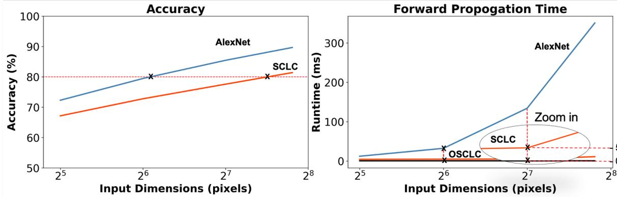
**FIGURE 4.** Accuracy and Forward propagation time for classification task on High-10 dataset. Left: AlexNet and SCLC accuracy for varying input resolution; Right: Forward propagation runtime of AlexNet, SCLC, and OSCLC for varying input resolution.
