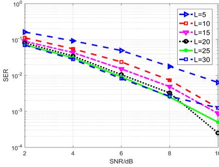
**Fig. 1.** The SER performances of the ADMM-HNet for a 16-QAM,  $M = 64$ ,  $K = 16$  for different number of layers.
