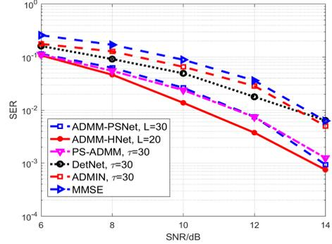
**Fig. 3.** The SER performance comparison for a 64-QAM,  $M = 64$ ,  $K = 16$ .
