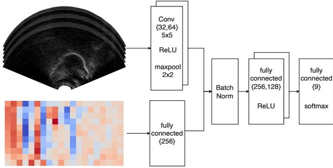
Figure 7: Convolutional neural network architecture for classifier using ultrasound and audio (MFCCs) inputs.
