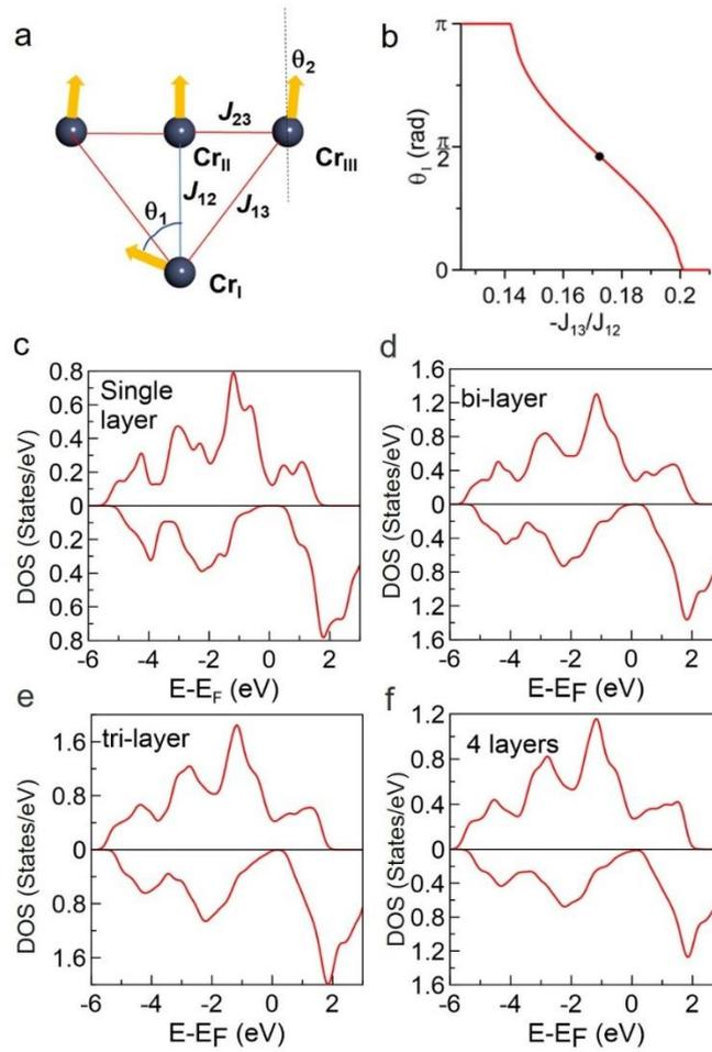
**Figure 3. Competition of spin exchange, spin canting and spin-resolved total density of states (DOS).** **a**, Schematic representation of exchange coupling in  $\text{Cr}_2\text{Te}_3$ . Competing inter-layer exchange parameters  $J_{12}$  and  $J_{13}$  induce canting angles  $\theta_1$  for  $\text{Cr}_I$  and  $\theta_2$  for  $\text{Cr}_{III}$  atoms. **b**,  $\theta_1$  as a function of the ratio of next-nearest to nearest
