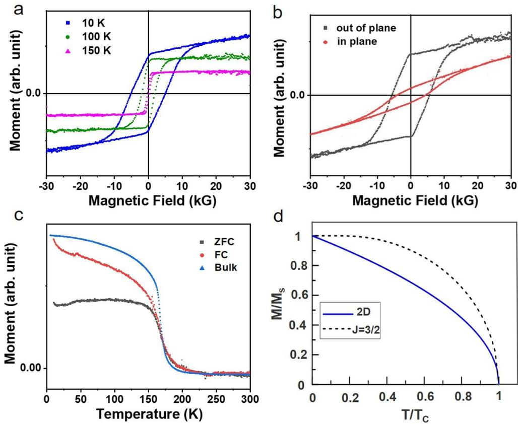
**Figure 4.** **a**, Out-of-plane magnetic hysteresis loops measured at different temperatures. **b**, Out-of-plane and in-plane magnetic hysteresis loops acquired at 10 K. **c**, ZFC and FC magnetization curves. The FC magnetization of a bulk film is also included for comparison. **d**, Calculated reduced magnetization as a function of reduced temperature of 2D (blue) compared to its 3D counterpart ( $J=3/2$ , black) in the mean field approximation.
