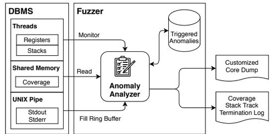
Fig. 5. Interaction between the anomaly analyzer and DBMS.
