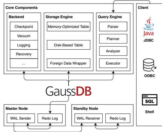
Fig. 1. Interactions between different processes/threads in GaussDB.
