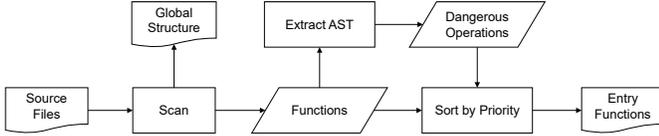
Fig. 2: *IntelliGen*’s process for locating entry functions.
