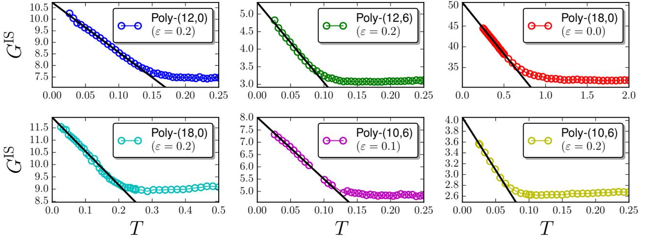
FIG. 5. Plot of inherent-state shear modulus  $G^{\text{IS}}$  as a function of temperature  $T$ . Black line is a linear fit to the low- $T$  portion of the data. Note that  $G^{\text{IS}}$  also exhibits a high- $T$  plateau-like regime.
