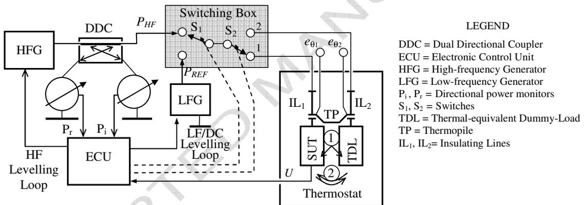
Figure 3. Quasi-true twin-microcalorimeter working configuration: the instrumentation set-up
