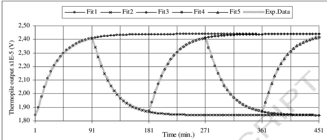
Figure 2. Extrapolated thermopile output waveform resulted by nonlinear fitting law method applied in the accelerated-measurements case for time constants  $\tau_1 = 29$  min. 4 s and  $\tau_2 = 4$  min. 28 s, a switching time  $T_S = 90$  minutes and an extrapolation time interval of 305 minutes.
