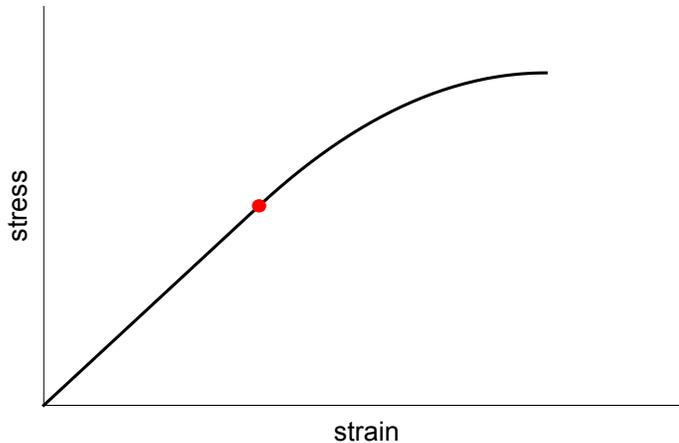
Figure 3: Idealised stress-strain behaviour of an individual collagen fibril stretched to failure. The fibril exhibits a linear response initially, before experiencing a decrease in gradient. Stretching beyond the linear region causes the fibril to become damaged [5], leading us to refer to the transition between linear and non-linear behaviour as the fibril yield stretch/strain, represented above by the red marker.
