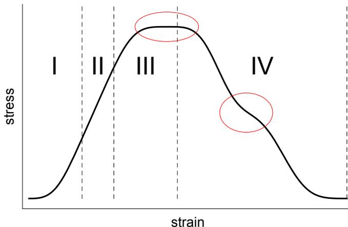
Figure 2: An idealised stress-strain curve demonstrating observed features (highlighted in red) which cannot be captured using existing models [1, 2]. Regions I and II are the same as in Figure 1, but the post-yield region (region III) shows a plateau instead of a well-defined peak. The macroscopic failure region (region IV) contains step-like failure behaviour, where the second derivative of the stress changes sign multiple times.
