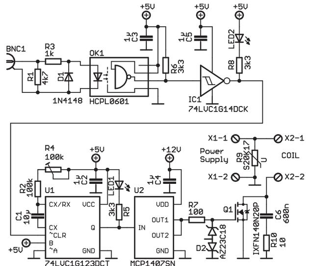
FIG. 3. Schematic of the control circuit of the fast coil.
