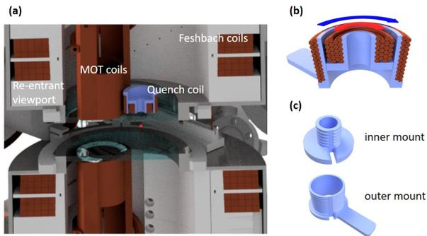
FIG. 1. Experimental setup and coils. (a) Schematic drawing of the metallic vacuum chamber and magnetic field coils. The red dot indicates the atoms in the chamber. (b) Design of the fast coil. The blue and red arrows show the current through the coils. (c) CAD drawing of the 3D printed mount of the coils.
