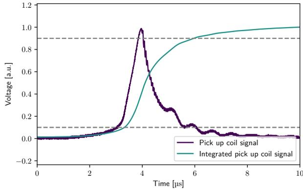
FIG. 4. Fast change of the magnetic field of the fast coil. The pick-up signal (purple) and its integrated signal (blue) during the magnetic field switching, the dashed lines indicate 10% and 90% voltage levels of the integrated signal. The time of the magnetic field change is about  $3 \mu\text{s}$ .
