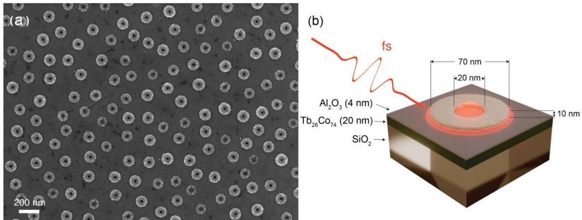
**Figure 1.** (a) SEM overview of the Ag nanoring antennas macroscopic assembly on a Tb<sub>26</sub>Co<sub>74</sub> film; (b) A schematic of the nanorings + ferrimagnetic film system (indicating the thicknesses /
