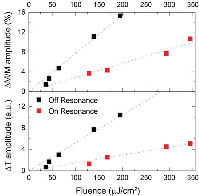
**Figure 4.** Degree of demagnetization (top panel) and maximum change in transmission (bottom panel) plotted as a function of incident fluence for resonant (red squares) and off-resonant pumping (black squares). The dashed lines are the corresponding linear fits to the data points.
