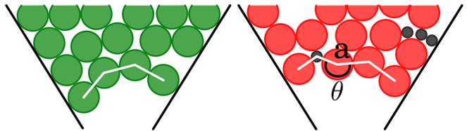
FIG. 3: Snapshots from a simulations with original particles (left) and with added particles of  $r = 0.4$  (right). These are long-lasting arches (more than 5 s) that needed to be removed. The branch vectors of the particles forming each arch are indicated with white segments. The large particle (indicated as “a”) presents branch vectors with angle  $\theta > 180$  Degree due to the neighboring small particle. This makes it especially unstable against vibrations [3].
