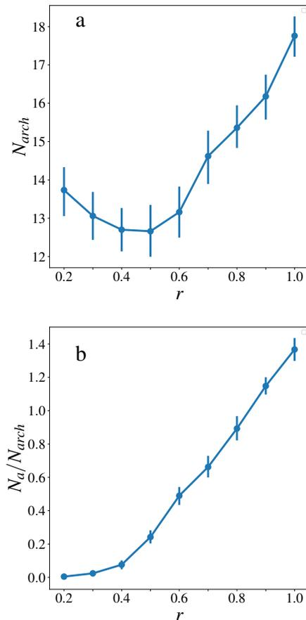
FIG. 5: (a) Number  $N_{arch}$  of long lasting arches that block the aperture as a function of  $r$  for  $\chi = 0.4$ . Long lasting means  $\tau > 5$  s. The error bars correspond to the standard deviation over 50 realizations. (b) Number  $N_a$  of small added particles per arch in long lasting arches ( $\tau > 5$  s) as a function of  $r$  for  $\chi = 0.4$ .
