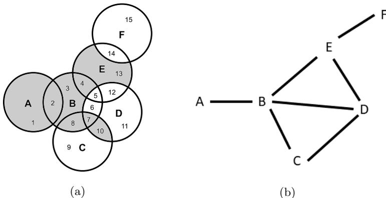
Figure 2: (a) Example with the primitives  $P = \{A, B, C, D, E, F\}$  and  $S$ , the solid to represent, in grey. The numbers 1-15 identify the non-empty fundamental products. (b) The corresponding intersection graph  $G$ . The example is adapted from [7].
