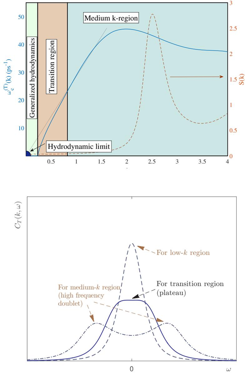
Figure 1: **Top:** Schematic illustrating the dispersion law of similar transverse acoustic oscillations  $\omega_c^{(T)}(k)$  and the static structure factor  $S(k)$  of some equilibrium liquid. **Bottom:** Schematic showing the form of the spectrum of the transverse current  $C_T(k, \omega)$  for the domain of intermediate values of the wave number  $k$ , for transition regime, and for the domain of generalized hydrodynamics (the small- $k$  limit).
