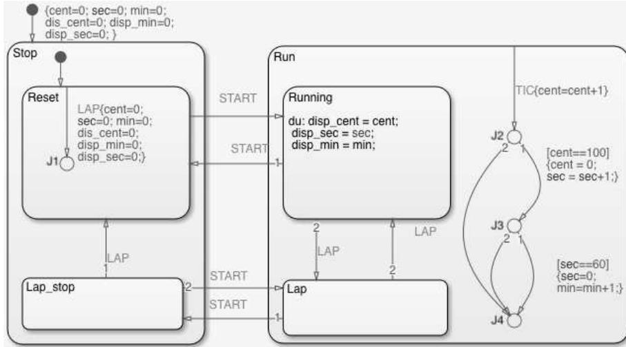
Figure 1: Simple Stateflow diagram - timer example [8].
