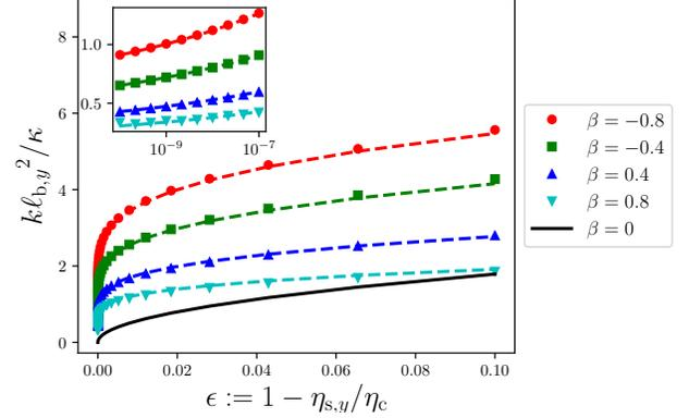
FIG. 4. Critical behavior of the indentation stiffness as  $\eta_c$  is approached, for five spheroidal geometries. Symbols denote data obtained from numerical integration of the stiffness integral. Solid and dashed lines correspond to analytical expressions Eqs. (3.8) and (3.15), respectively. Inset shows the same data on linear-log scales to reveal the slow approach to zero stiffness as  $\eta_{s,y} \rightarrow \eta_c^+$  for non-spherical shells.
