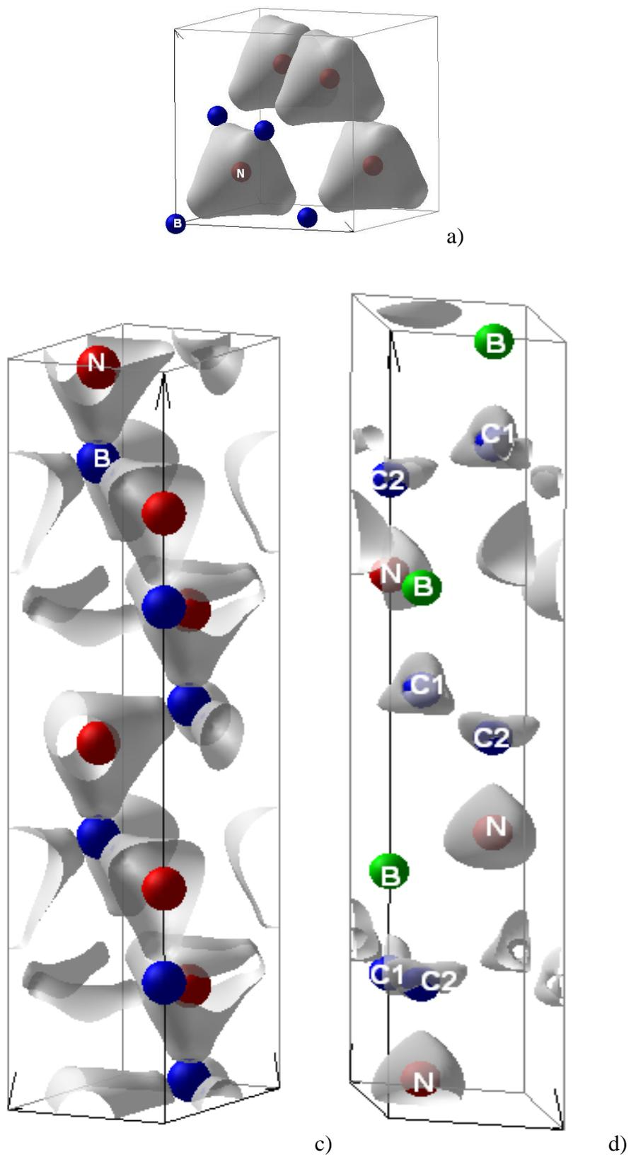
Fig. 2 Charge density isosurfaces of 3D phases: a) *c*-BN, c) *h*-B<sub>6</sub>N<sub>6</sub> and d) *h*-B<sub>3</sub>C<sub>6</sub>N<sub>3</sub>.
