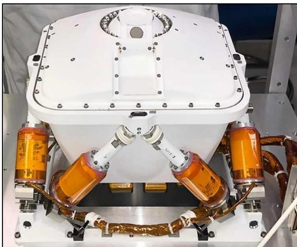
**Fig. 1:** The PIXL sensor assembly prior to integration on the rover arm turret.
