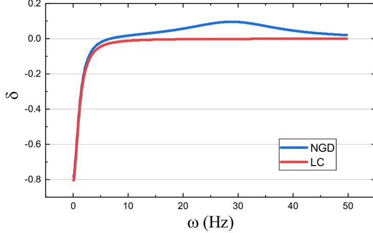
FIG. S1: Group delay from the two models. Parameters for the NGD model are:  $\alpha = 20s^{-1}$ ,  $\beta = 1.22s^{-1}$  and  $kg = 920s^{-2}$  while  $\lambda = 0.45$  in the LC model. These parameters meet the two conditions so that two models can be related by  $\lambda = (1 + \beta)^{-1}$  at low  $\omega$ .
