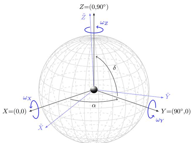
**Fig. 2.** The ICRF is modeled as an orthogonal vector triad  $\mathbf{C} = [\mathbf{X} \ \mathbf{Y} \ \mathbf{Z}]$ . The transformation from  $\mathbf{C}$  to  $\hat{\mathbf{C}} = [\hat{\mathbf{X}} \ \hat{\mathbf{Y}} \ \hat{\mathbf{Z}}]$  is obtained by applying the spin  $\boldsymbol{\omega} = [\omega_X \ \omega_Y \ \omega_Z]$ , which is a combination of rotations around the axes  $\mathbf{X}$ ,  $\mathbf{Y}$ , and  $\mathbf{Z}$ .
