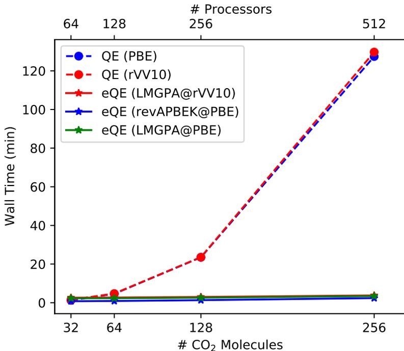
Figure 2: Wall times when simulating supercells containing 32, 64, 128, and 256 CO<sub>2</sub> molecules. The corresponding numbers of MPI tasks are 64, 128, 256, 512. Full lines are eQE simulations with different NAXE functionals. Dotted lines are KS-DFT (QE version 6.6) simulations for the same systems and same cutoff for the plane waves (i.e., 40 Ry for the wavefunctions and 400 Ry for the electron density).
