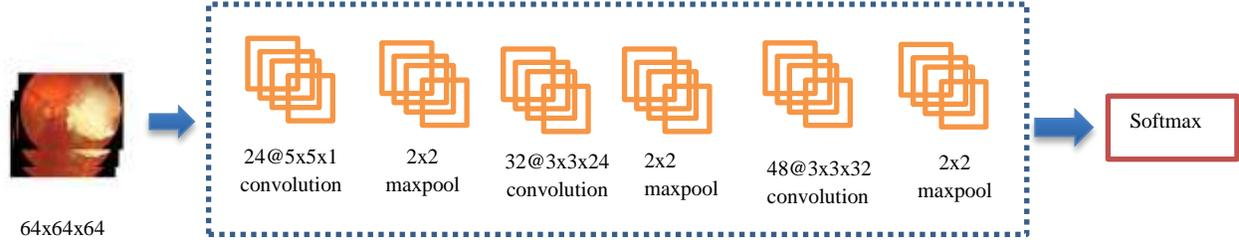
**Figure 6** The proposed 2.75D CNN Architecture.
