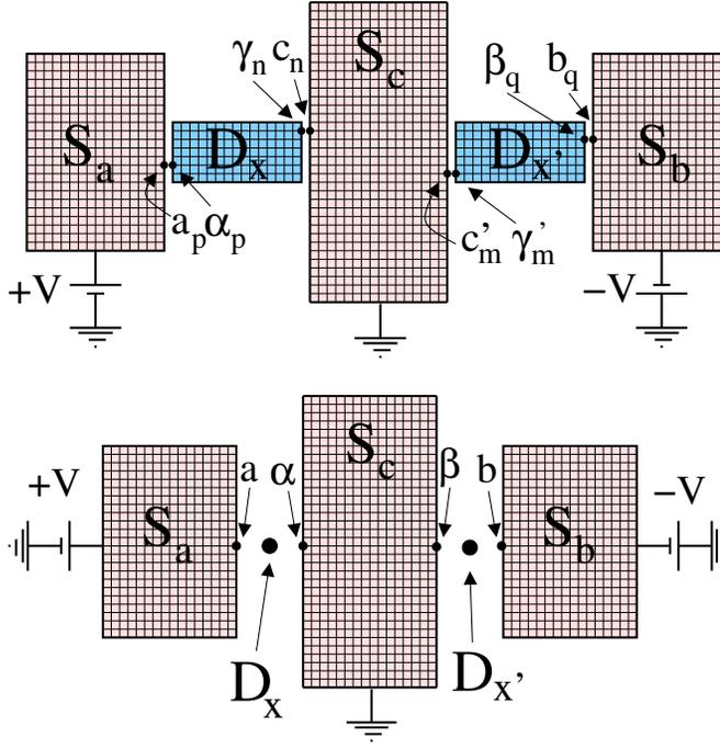
FIG. 5. Schematic tight-binding model of the considered  $S_a$ - $D_x$ - $S_c$ - $D_x'$ - $S_b$  three-terminal Josephson junction containing two quantum dots  $D_x$  and  $D_x'$ . The quantum dots have finite dimension on this figure. This is "the model I".
