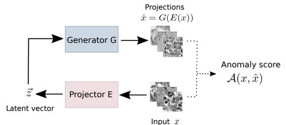
**Fig. 1.** Scheme of GAN-based unsupervised anomaly detection. The original input image  $x$  is fed through projector  $E$  which outputs a latent vector  $z$ . This latent vector is used to generate a reconstruction image via generator  $G$ . An anomaly score is a measure of some difference between the input image  $x$  and its reconstruction  $\hat{x}$ .
