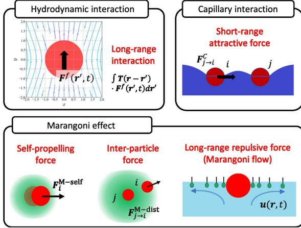
FIG. 1. Five physical mechanisms introduced in our model; long-range hydrodynamic interaction (RPY type mobility tensor with mirror image method applied), short-range capillary interaction, self-propelling force induced by the Marangoni effect, short-range interaction due to the concentration field of surfactant, and Marangoni flow that produces long-range repulsive force.
