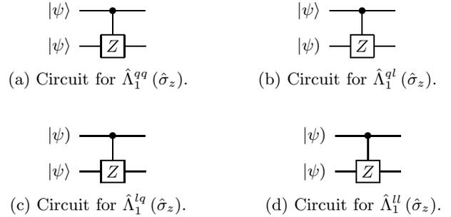
FIG. 3: Four different controlled-Z gates
