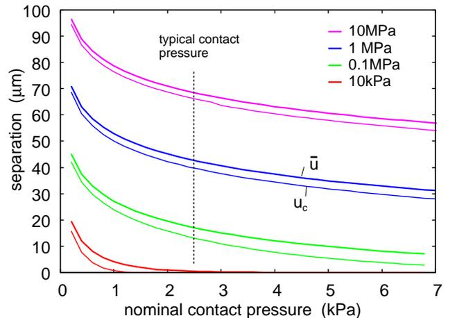
FIG. 10. The average interfacial separation  $\bar{u}$ , and the separation  $u_c$  which determines the air leakage [see (4)], as a function of the nominal contact pressure. Results are shown for the elastic modulus  $E = 10, 1, 0.1$  and  $0.01$  MPa. In all cases the Poisson ratio  $\nu = 0.5$ . Only the surface roughness of the skin (with the power spectrum shown in Fig. 2) is included in the calculations.
