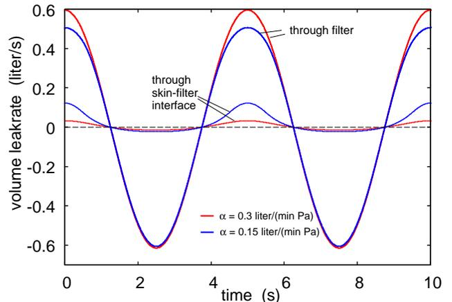
FIG. 3. The air (of atmospheric pressure) volume leak rate in liter/s as a function of time during breathing at the period of  $T = 5$  sec and the volume  $V_0 = 0.5$  liter:  $V(t) = V_0 \sin(\omega t)$  with  $\omega = 2\pi/T$ . The red and blue curves are for the filter air flow conductance  $\alpha = 0.3$  and 0.15 liter/(min  $\cdot$  Pa). The thick lines is the leakage through the filter and the thinner lines at the skin-filter interface.
