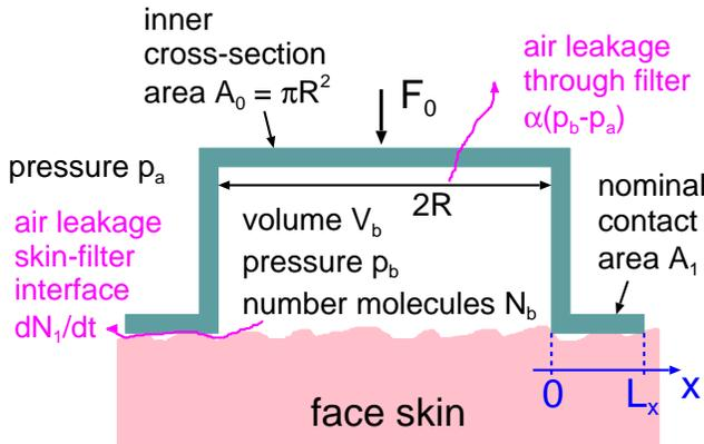
FIG. 1. Model used for studying the air flow for facemask. The air can flow through the filter at a number flow rate  $\alpha'(p_b - p_a)$  or at the interface between the skin and the facemask at a number flow rate  $dN_1/dt = \dot{N}_1$ . The number of air molecules  $N_b$  and the air pressure  $p_b$  in the volume  $V_b$  between the facemask and the face varies in time due to the breathing act.
