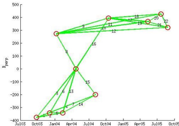
Fig. 3. The SBAS network derived from the time series analysis: vertical and horizontal axes indicate the perpendicular and temporal baselines, respectively.
