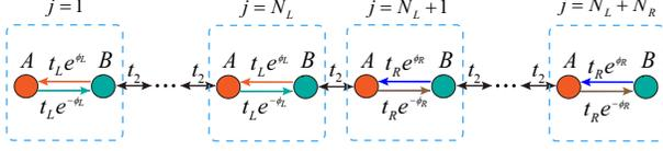
FIG. 3. Schematic of a non-Hermitian SSH model under the domain-wall configuration. The intra-cell hopping from sublattice sites  $a$  to  $b$  in the left(right) bulk is  $t^{L(R)} e^{\phi_{L(R)}}$ , while the intra-cell hopping from  $b$  to  $a$  is  $t^{L(R)} e^{-\phi_{L(R)}}$ . For simplicity, we assume both bulks have the same  $t_2$ .
