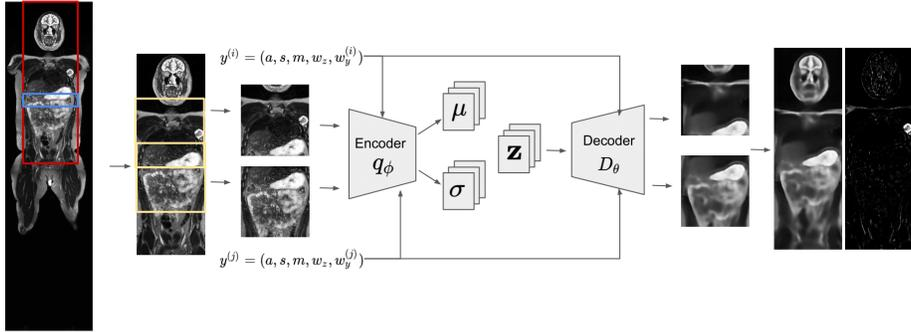
**Fig. 1.** Framework overview. The blue bounding box is determined by multi-scale template matching and determines the width of the chest. The red box then defines the region of interest. Square windows (yellow) within the region of interest are inputted to the spatial VAE.
