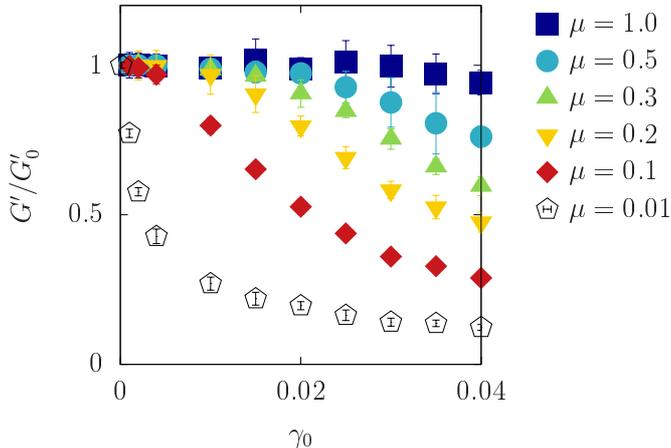
**Fig. 7** Plots of the normalized storage modulus  $G'/G'_0$  versus  $\gamma_0$  for various  $\mu$  values.
