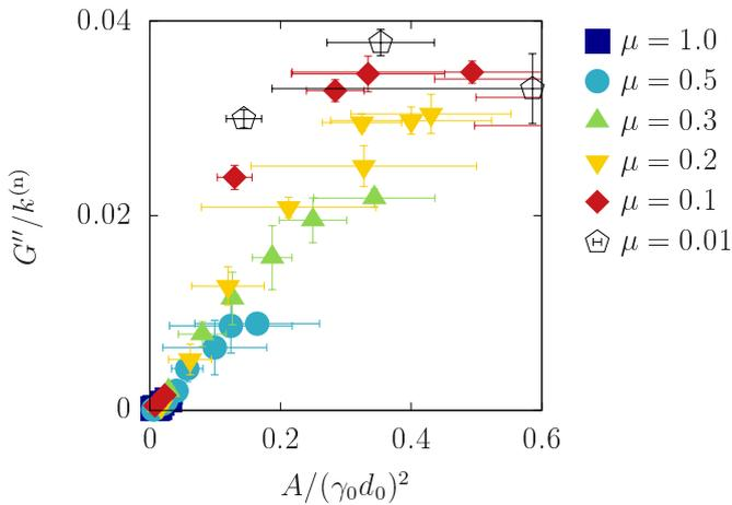
**Fig. 11** Plots of the loss modulus  $G''$  versus  $A/(\gamma_0 d_0)^2$  for various values of  $\gamma_0$  and  $\mu$ .
