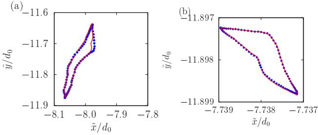
**Fig. 3** Non-affine particle trajectories for  $\gamma_0 = 0.04$  (a) and  $0.004$  (b) with  $\mu = 0.1$ . The circles represent the trajectory in the last cycle. The line represents the trajectory in the second to the last cycle.
