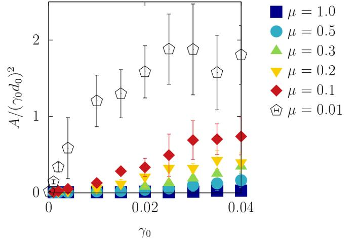
**Fig. 6** Plots of the normalized area  $A/(\gamma_0 d_0)^2$  of loop trajectories versus  $\gamma_0$  for various values of  $\mu$ .
