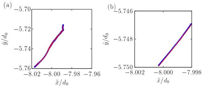
**Fig. 5** Non-affine particle trajectories for  $\gamma_0 = 0.04$  (a) and  $0.004$  (b) with  $\mu = 1.0$ . The circles represent the trajectory in the last cycle. The line represents the trajectory in the second to the last cycle.
