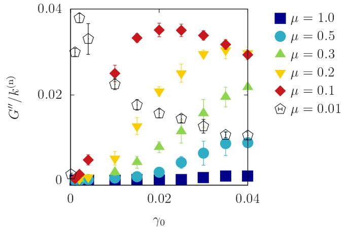
**Fig. 9** Plots of the loss modulus  $G''$  versus  $\gamma_0$  for various values of  $\mu$ .
