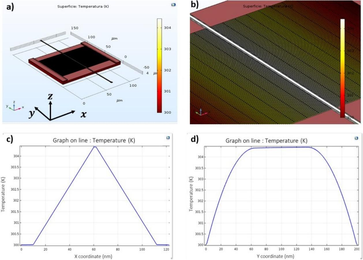
FIG. 3. FEM simulation results. Panel a): FEM simulation of temperature distribution for the device sketched in the figure 2. Panel b): FEM simulation of temperature distribution (enlargement of the device). Panel c): temperature trend along the nanostructures ( $x$  axis). Panel d): temperature trend along the central silicon ribbon ( $y$  axis), where there is the metal track acting as heater generator.
