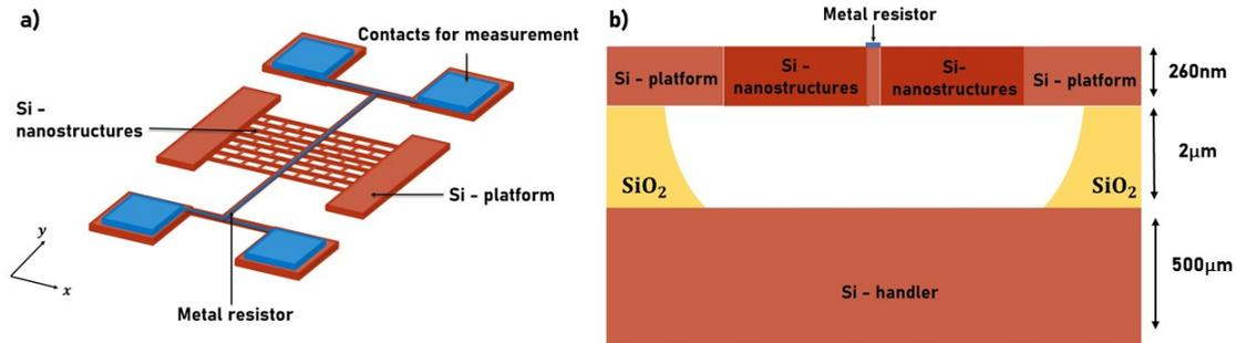
FIG. 2. Sketches of the device. Panel a): an overall vision of the device. Panel b): a cross section in  $x$  direction, showing the suspended nanostructures.
