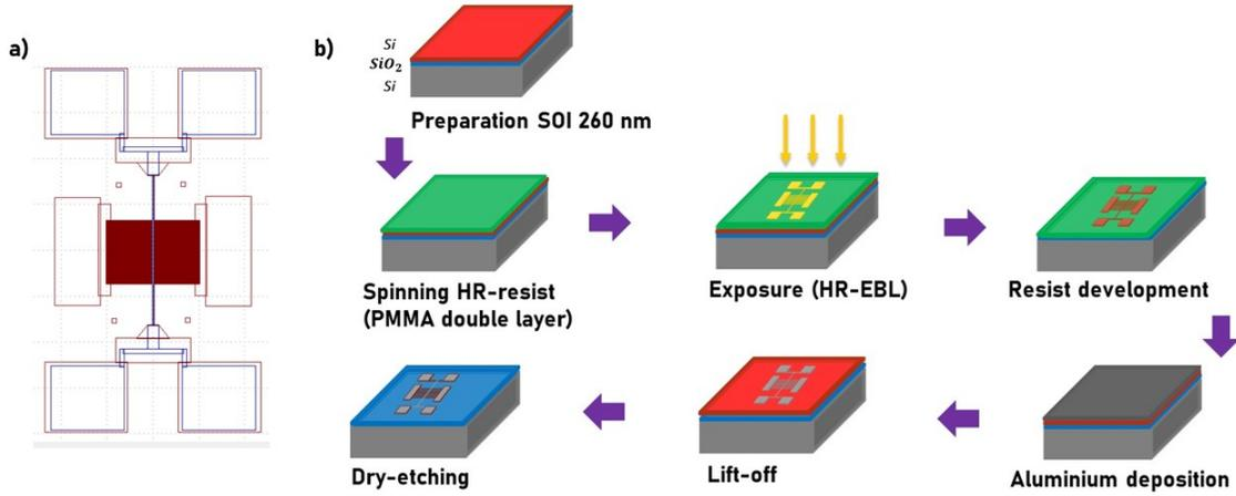
FIG. 4. Panel a): mask design of the device: red geometries represent the layout of the nanostructures, blue geometries represent the metal track and the pads for the external connections. Panel b): sketches of the process steps for the fabrication of the device.
