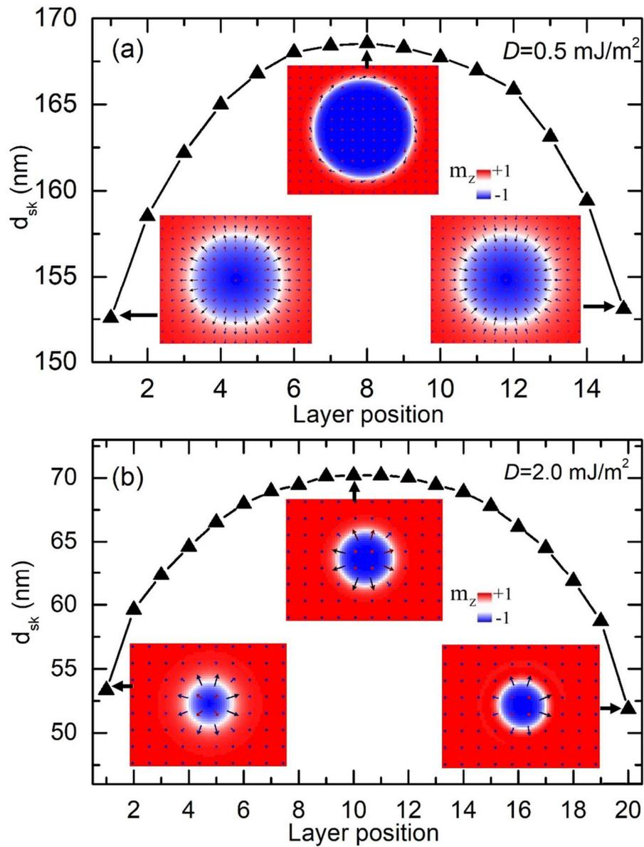
Figure 2: Micromagnetic simulations of skyrmion textures in low and high DMI systems. Skyrmion diameter as a function of layer position for (a) Pt/Co/MgO at  $H_{ext}=110 \text{ mT}$  and (b) Fe(0.4)/Co(0.4) at  $H_{ext}=160 \text{ mT}$ . The insets depict the spatial distribution of the skyrmion magnetization at the layer positions indicated by the black arrows. The colors correspond to the normalized z-component of the magnetization, as shown in the color bar.
