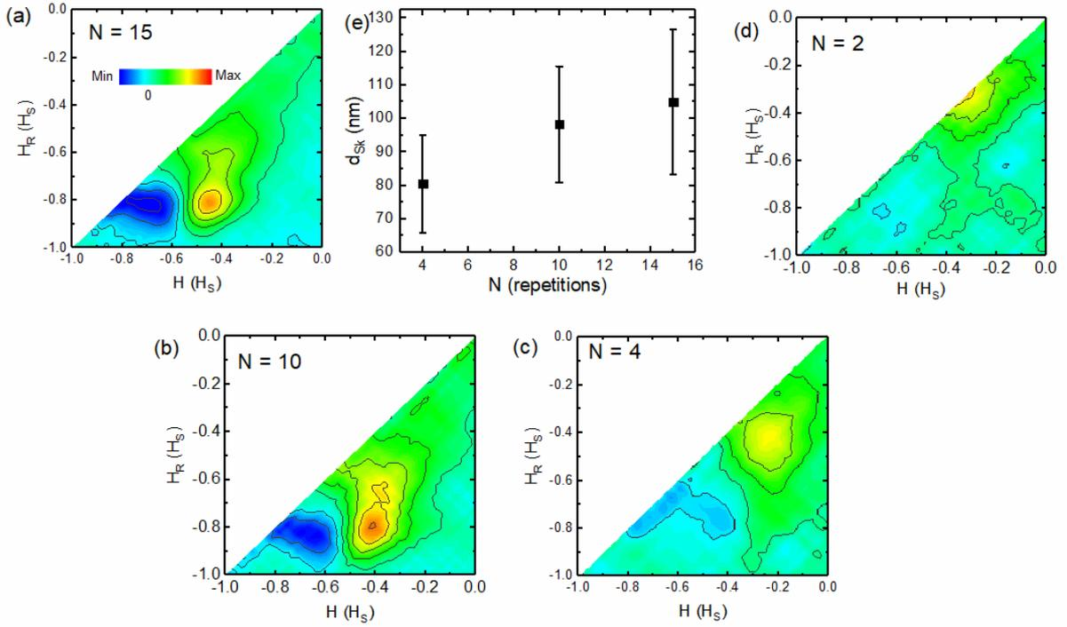
Figure 3: Evolution of FORC distributions with number of layer repetitions ( $N$ ) in Pt/Co/MgO multilayers
