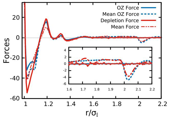
FIG. 3. Depletion (solid lines) and mean (dashed lines) forces, times  $\beta\sigma_l$ , between large particles for a system with  $\phi = 0.55$ , having  $\phi_l = 0.4$ ,  $\phi_m = 0.075$ , and  $\phi_s = 0.075$ . The red lines were obtained using the procedure presented in this letter; the blue lines with the integral equations approach for the depletion forces [7]. Mean OZ force stands for the mean force obtained from the  $g(r)$  resulting from the solution of the OZ equation.
