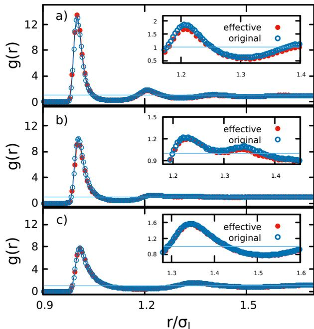
FIG. 2. Radial distribution functions between large particles for the three systems in Fig. 1. Insets show closer details around the second minimum. The blue circles are the simulations results for the original mixture with the bare interactions and the red circles the simulations results for the effective monodisperse system of large particles interacting with the depletion forces shown in Fig. 1.
