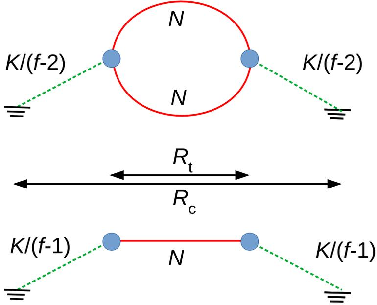
Figure 2: Comparison of a loop made of two strands,  $i = 2$ , (top part) with a network strand in the ideal tree approximation (lower part). The red lines indicates the real strands, the green dashed lines are the virtual strands that connect to the non-fluctuating elastic background (or to ground in the resistor analogy).  $R_t$  and  $R_c$  are the time average size of the real strands and the combined strand respectively.
