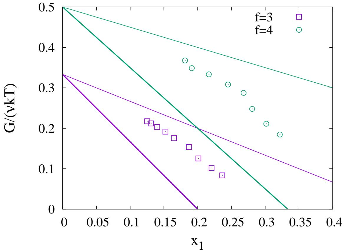
Figure 3: Comparison of the loop dependence of modulus data of Ref.<sup>5</sup> with the lower bound of equation (13) as shown by the thick lines, while the thin lines indicate the corrections due to pending loops only,  $c_f = 1$ , which is equivalent to the estimate from the resistor analogy.
