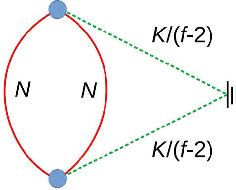
Figure 1: Resistor analog for a loop made of  $i = 2$  strands of  $N$  segments. The blue circles represent the junctions of the loop. The virtual strands of  $K/(f - 2)$  describe the effective connection to ground through the  $f - 2$  strands of  $K$  effective segments. See Ref.<sup>4</sup> for more details.
