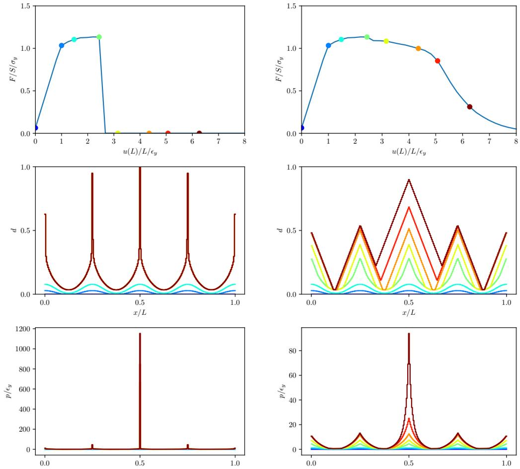
**Figure 11.** Response for a softening plasticity model with a volumic oscillatory force. No regularization,  $l = 0$  (left) and Lip regularization (right). Stress-average strain results (top), damage (middle) and cumulative plasticity profile (bottom). Parameters are:  $L = 1.$ ,  $l = 0.25$ ,  $h = 1/255$ ,  $E = 1.$ ,  $\sigma_y = 1/16$ ,  $k = 4$ .
