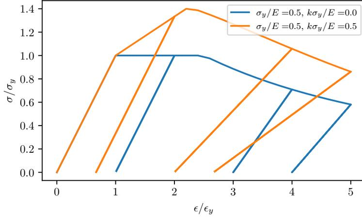
**Figure 4.** Stress-strain relations for the softening elasticity model with hardening plasticity with the choice  $\epsilon_c/\epsilon_y = 2$  where  $\epsilon_y = \sigma_y/E$ . The strain loading/unloading follows the peak value sequence  $\epsilon/\epsilon_y = (0, 2, e_1, 4, e_2, 5, e_3)$  where  $e_1, e_2, e_3$  indicate the strain needed to reach full unloading ( $\sigma = 0$ ).
