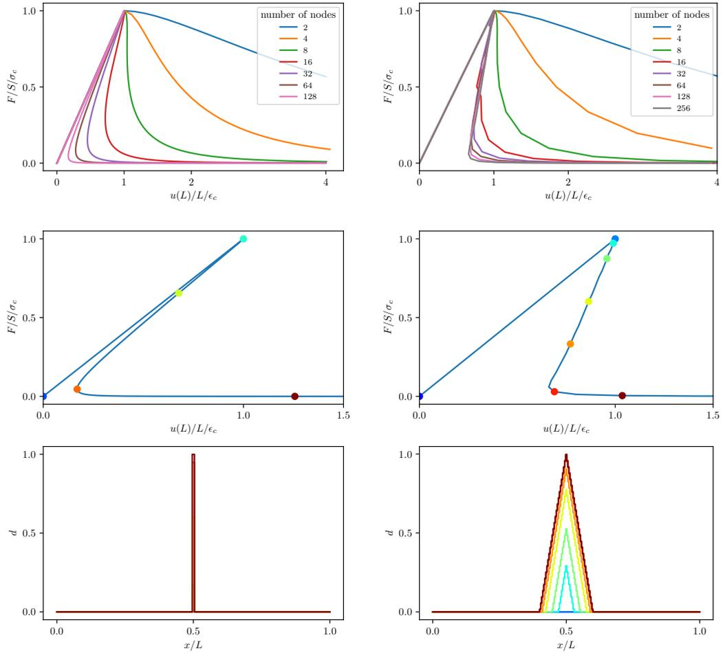
**Figure 8.** Response for the bar with the elastic softening behavior and snap-back control: non-regularized model (left) and Lip-field model (right), convergence of the stress-average strain response (top) and damage evolution (bottom) corresponding the color dots in the middle figures. The middle figures reproduce the curve of the top figures for the most refined grid. Parameters are:  $L=1$ ,  $l = 0.1$ ,  $E = 1$ ,  $Y_c = 1$ ,  $\lambda = 0.3$ ,  $G_c = 2/3$ .
