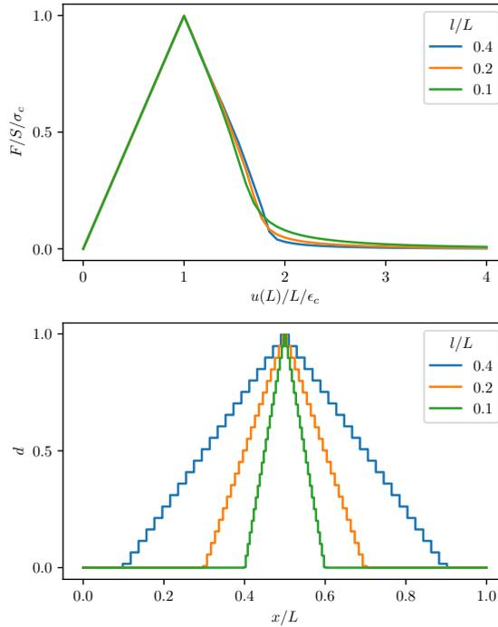
**Figure 9.** Lip-field model response with the elastic softening behavior (choice  $h_2$ ) for several regularization length values. Stress-average strain response (above) and damage profile (below). Parameters are:  $L = 1$ ,  $l = (0.4, 0.2, 0.1)$ ,  $E = 1$ ,  $Y_c = 1$ ,  $\lambda = (0.4, 0.2, 0.1)$ ,  $G_c = 2$ . The number of elements is 51, 101 and 201 so that we have  $h/l \sim 20$ .
