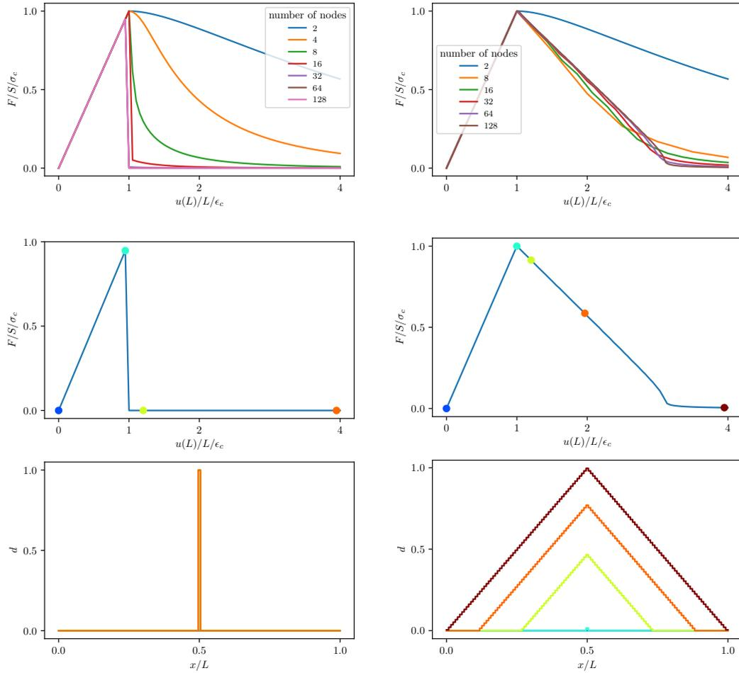
**Figure 7.** Response for the bar with the elastic softening behavior and imposed displacement: non-regularized model (left) and Lip-field model (right). The top row gives the stress-strain average response and the bottom one the damage profile at the color dots given in the middle row. The mesh used for the middle row is the most refined of the top row. Parameters are:  $L=1$ ,  $l = 0.5$ ,  $E = 1$ ,  $Y_c = 1$ ,  $\lambda = 0.3$ ,  $G_c = 10/3$ .
