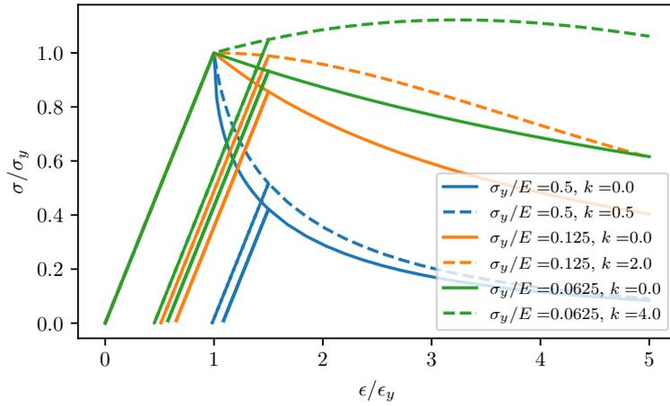
**Figure 5.** Stress-strain relations for the softening plastic model ( $\epsilon_y = \sigma_y/E$ ). The strain loading/unloading follows the peak value sequence  $\epsilon/\epsilon_y = (0, 1.5, e, 5)$  where  $e$  indicates the value needed to reach  $\sigma = 0$ .
