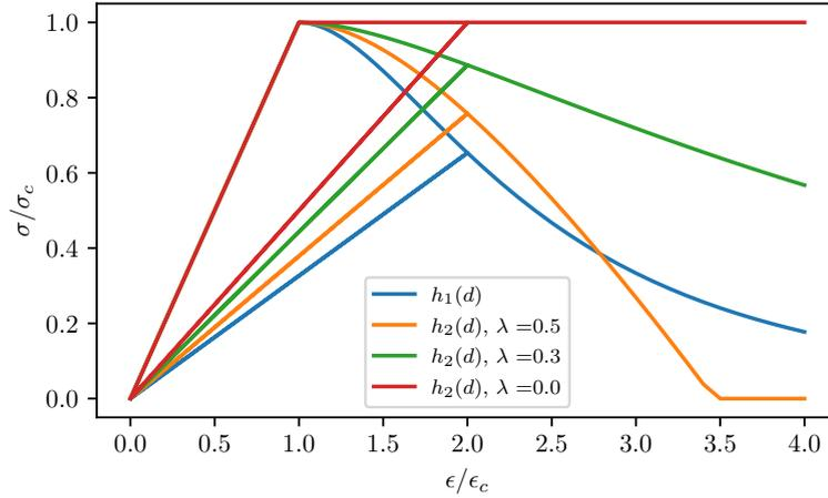
**Figure 3.** Stress-strain relations for the softening elastic model ( $\sigma_c = \sqrt{2EY_C}$ ,  $\epsilon_c = \sigma_c/E$ ). The strain loading/unloading follows the peak values sequence:  $\epsilon/\epsilon_c = (0, 2, 0, 4)$ .
