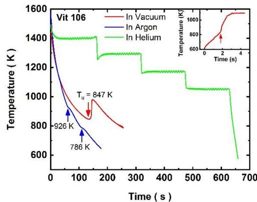
Fig. 1. Typical time-temperature plots during cooling of a Vit106 ( $Zr_{57}Cu_{15.4}Ni_{12.6}Al_{10}Nb_5$ ) liquid under vacuum, Ar- and He-atmospheres. Complete and partial crystallizations happened in vacuum and under Ar-atmospheres. The arrows indicate the crystallization events. Crystallization was completely suppressed in He-atmosphere due to a much faster cooling. The inset shows the recalescence rise in temperature when the glass transformed into crystals during the next heating cycle.
