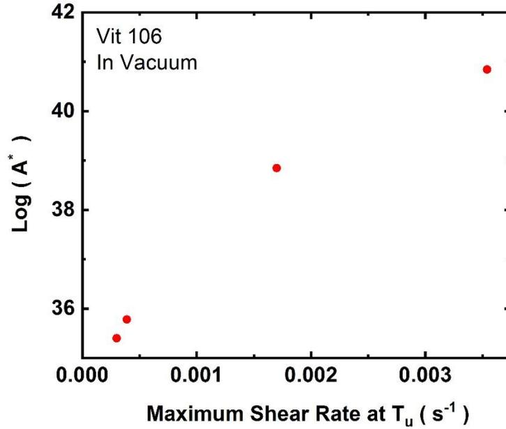
Fig. 2. The prefactor  $A^*$  for nucleation as a function of the maximum shear rate at the nucleation temperature ( $T_u$ ) for processing in vacuum for liquid Vit106 ( $Zr_{57}Cu_{15.4}Ni_{12.6}Al_{10}Nb_5$ ). The nucleation temperatures and the relevant parameters are presented in tables 1.
