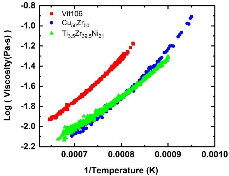
Fig. S.1. The viscosities of three different liquids as a function of temperature measured by the ESL technique.
