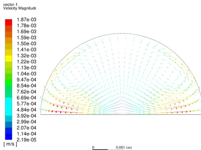
Fig. S.2. The fluid flow velocity distribution in a 6.0 mm diameter  $\text{Ti}_{39.5}\text{Zr}_{39.5}\text{Ni}_{21}$  liquid at 990 K when the sample was cooled with a 5.7 V positioner and heater off condition. As is apparent from the color code, the flow velocities are maximum at the equator and minimum at the poles.
