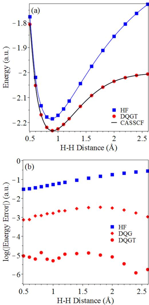
FIG. 1. The (a) total energy and the (b) energy errors of the potential energy curve of the  $H_4$  chain are shown for its equally spaced dissociation in a [4,4] active space in the cc-pVQZ basis set. Errors are relative to CASSCF. The variational 2-RDM energies with the DQG and DQGT conditions agree with those from CASSCF to about  $10^{-3}$  a.u. and  $10^{-5}$  a.u., respectively.
