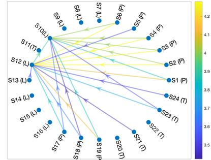
Fig. 6. Causality graph in oil and gas plant estimated by NL-TISO
