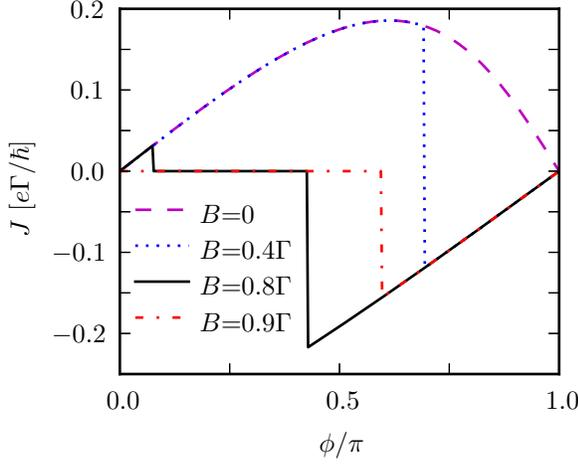
FIG. 2. Josephson current  $J$  as a function of the phase  $\phi$  for different values of the magnetic field  $B$  and vanishing coupling to the oscillator,  $\lambda = 0$ . Parameters are  $\epsilon = -U_C/2$ ,  $t = U_C = \Gamma$ , and  $k_B T = 0$ .
