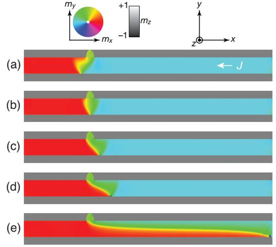
FIG. 2. Static domain wall profiles under different applied dc currents,  $J(t) = J_0$ . (a)  $J_0 = -4$ , (b)  $J_0 = 0$ , (c)  $J_0 = 4$ , (d)  $J_0 = 8$ , and (e)  $J_0 = 10$  TA/m<sup>2</sup>. The critical depinning current is approximately  $J_{0,c} = 8.5$  TA/m<sup>2</sup>. The functionality of the DWMGO is limited to currents below this critical current.
