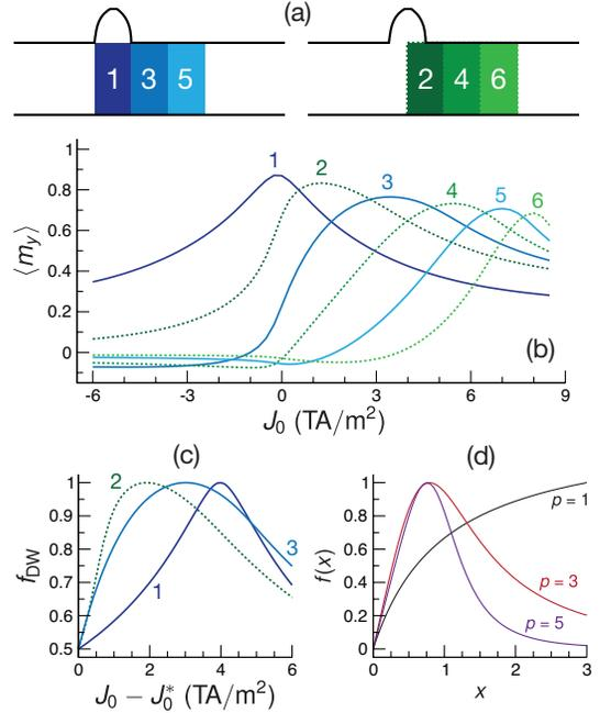
FIG. 3. Magnetoresistive readout signal of the DWMGO. (a) Example of six sensor positions. (b) Spatial average of  $m_y$  as a function of the static applied current  $J_0$  for each sensor position in (a). (c) Rescaled output function at the operating point of sensor positions 1 to 3. (d) Mackey-Glass transfer function for three different  $p$  for comparison.
