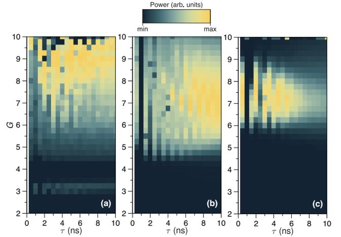
FIG. 7. Phase diagram of the output power of the oscillator as a function of feedback delay,  $\tau$ , and gain,  $G$ , for the readout sensor located at (a) position 1, (b) position 2, and (c) position 3.
