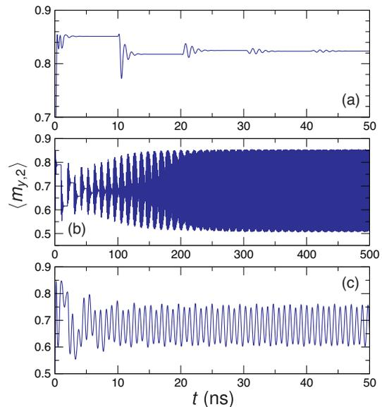
FIG. 4. Time traces of the magnetization dynamics measured at Position 2. (a) Transient dynamics toward a static configuration under weak amplification,  $G = 2$ , and long delays,  $\tau = 10$  ns. (b) Self-sustained oscillations at  $G = 6$  and long delays,  $\tau = 10$  ns. Self-sustained oscillations at  $G = 6$  and short delays,  $\tau = 1$  ns.
