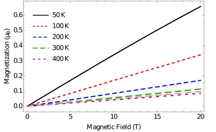
Figure S2. Magnetization  $\mathcal{M}_z$  as a function of the magnetic field  $B_z$  for the temperature range under which the magnetic susceptibility of the described metal complex is measured. As can be seen, in the entire temperature range the system remains in the regime of magnetic susceptibility (linear magnetization) up to dozens of Tesla.
