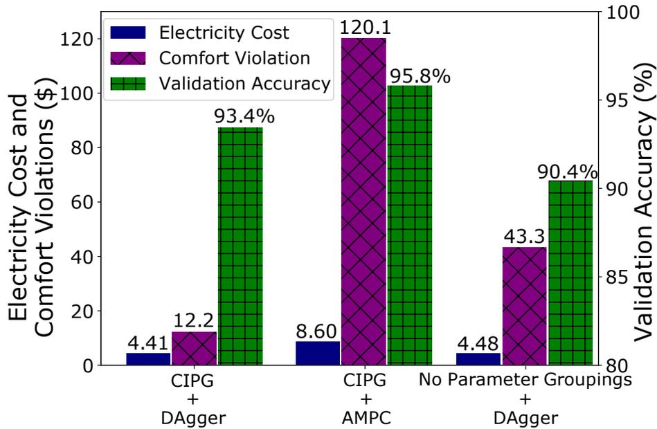
Figure 3: Per-unit Control Objectives (lower is better) and Validation Prediction Accuracy (higher is better) for (1) constraint informed parameter groupings (CIPG) with DAgger training data, (2) CIPG and trained to approximate closed loop MPC (AMPC), and (3) CIPG with DAgger training data. When combined, our contributions, CIPG and DAgger, provide more stability and lower costs.
