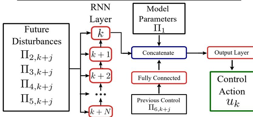
Figure 2: Reverse-Time Recurrent Neural Network Structure. Future disturbance parameter groupings containing weather, electricity price, and setpoint information are input into the reverse RNN layer where information flow backward in time over MPC horizon. These are concatenated with inputs from the other parameters and then to the output layer.
