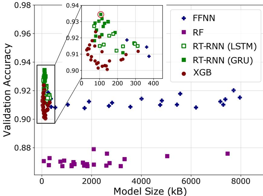
Figure 4: Validation accuracy versus model size for each of the four tested machine learning algorithms. The reverse-time RNN (RT-RNN) models largely outperform the other models on both metrics: It can maintain the highest prediction accuracy with a very small memory requirement. The circled marker denotes the chosen model.
