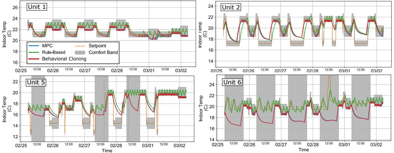
Figure 6: Test control plots for a representative sample of the buildings under each control method. Both MPC and Behavioral Cloning can more effectively take advantage of varying setpoint schedules and comfort bands by reducing consumption during times the resident is away, and optimally preheating to avoid comfort violations.
