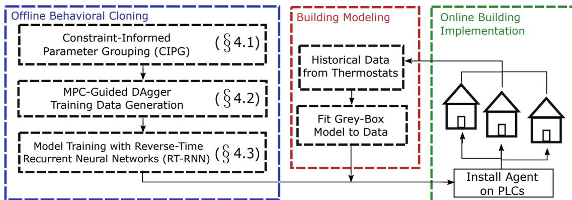
Figure 1: Overall methodology for Behavioral Cloning of MPC and implementing it in a population of buildings. Behavioral Cloning and building modeling can both be performed offline using a desktop computer, while online control only requires a programmable logic controller (PLC).
