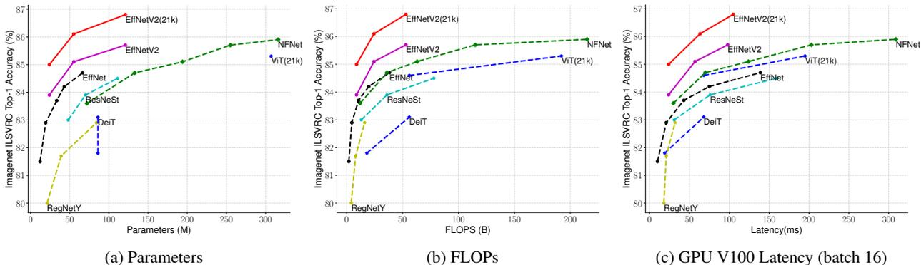
**Figure 5. Model Size, FLOPs, and Inference Latency** – Latency is measured with batch size 16 on V100 GPU. 21k denotes pretrained on ImageNet21k images, others are just trained on ImageNet ILSVRC2012. Our EfficientNetV2 has slightly better parameter efficiency with EfficientNet, but runs 3x faster for inference.
