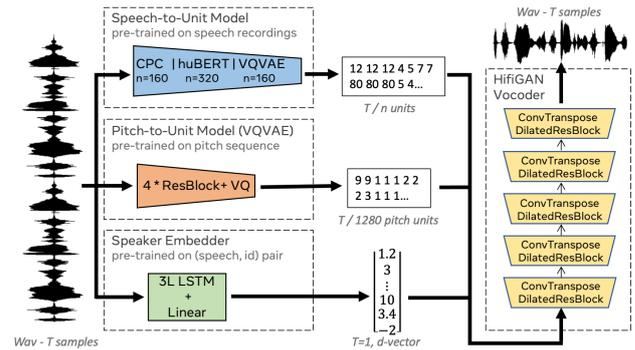
Figure 1: *The overall proposed speech resynthesis architecture. Three parallel encoders extract speech discrete representations from the raw input signal. These are then being used as a conditioning to reconstruct the signal using a decoder network.*
