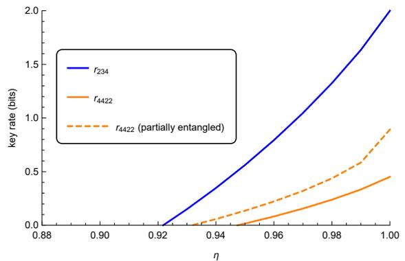
FIG. 1. Secret key rates versus detection efficiency  $\eta$ . Comparison between the secret key rate obtained with  $Q_{234}$  (blue line),  $Q_{4422}$  (solid orange line), and the realization described in Section II C (dashed orange line). The corresponding thresholds to distill a secret key are 0.9218, 0.9474 and 0.9317, respectively.
