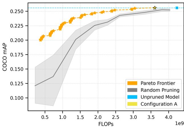
**Fig. 2. Accuracy and FLOPs trade-offs for different optimal anchor configurations found by our anchor pruning search. The Pareto frontier is highlighted in orange, the unpruned baseline in blue. Accuracy is measured on the COCO val2017 dataset and FLOPs indicate the multiply-adds in the detection head.**
