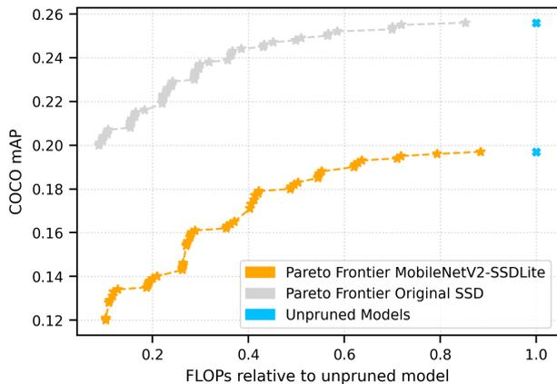
Fig. 6. Accuracy and number of FLOPs relative to the unpruned models for MobileNetV2-SSDLite and the original SSD on COCO val2017. Both frontiers have a similar trend line, indicating that anchor pruning is backbone agnostic.
