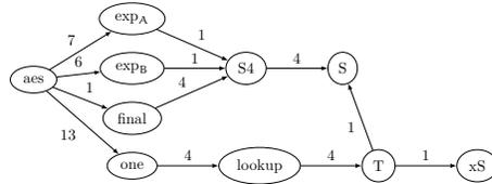
**Fig. 5:** Module dependency graph of the AES-256 benchmark.
