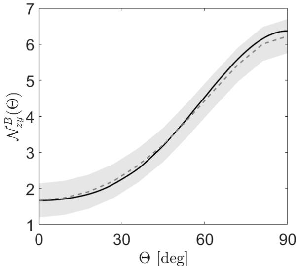
FIG. 2. The number of collisions per rethermalization  $\mathcal{N}_{zy}^B$  as a function of  $\Theta = 0-90$  (deg), obtained from the theory [Eq. (14)] (solid, black curve) and fits to  $\mathcal{T}_y$  from DSMC simulations using Eq. (13) (dashed-dotted, grey data) with error bars (filled, grey region). These results are with the parameters in Tab. I, and  $a = 39.8$  ( $a_0$ ).
