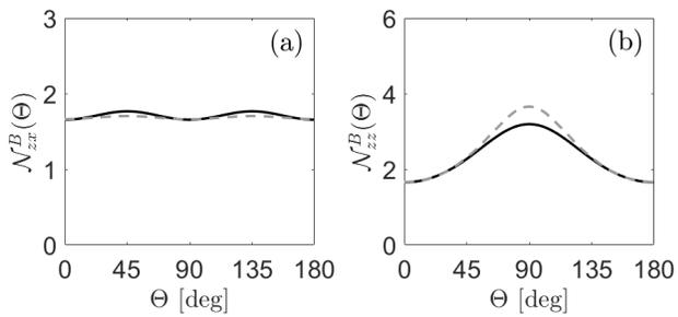
FIG. 5. The number of collisions per rethermalization (a)  $\mathcal{N}_{zx}^B$  and (b)  $\mathcal{N}_{zz}^B$  vs  $\Theta = 0$ –180 (deg), as computed using the short-time approximation (solid, black curve) and the full Enskog solution (dashed, grey curve). These results are with the parameters in Tab. I, and  $a = 39.8$  ( $a_0$ ).
