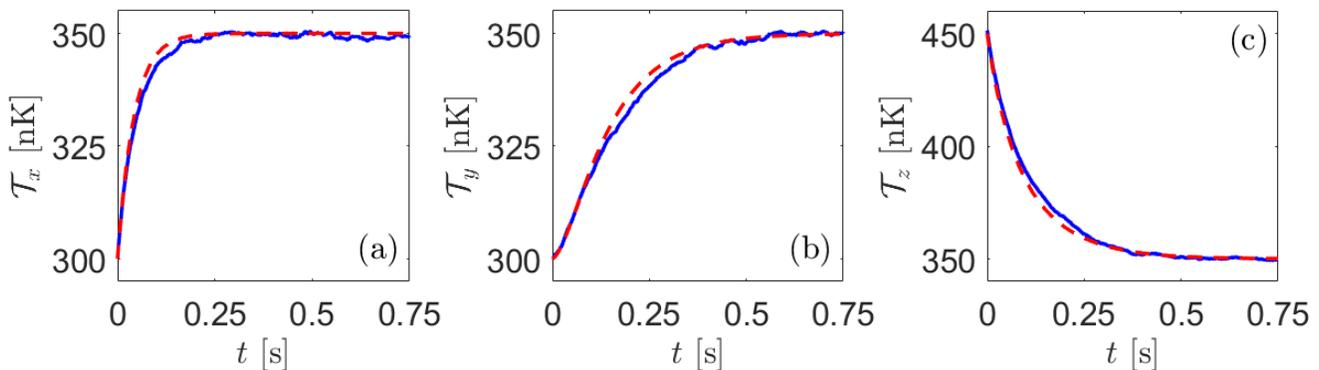
FIG. 1. Rethermalization curves of the pseudotemperatures (a)  $\mathcal{T}_x$ , (b)  $\mathcal{T}_y$  and (c)  $\mathcal{T}_z$ , with excitation along  $z$ , as generated by DSMC simulations (solid, blue) and solutions to the Enskog equations (dashed, red). Simulation parameters are those in Tab. I, with the scattering length is set to  $a = 39.8 (a_0)$  and  $\Theta = 90$  (deg).
