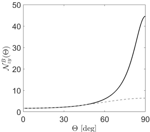
FIG. 3. The number of collisions per rethermalization,  $\mathcal{N}_{zy}^B$  vs  $\Theta = 0$ –180 (deg), as computed using the short-time approximation (solid, black curve) and the full Enskog solution (dashed, gray curve). These results are with the parameters in Tab. I, and  $a = 39.8$  ( $a_0$ ).
